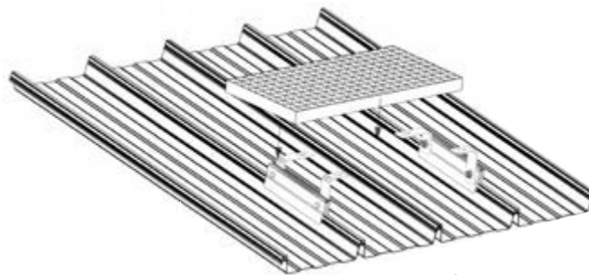
Tread supports RIB-ROOF 465
