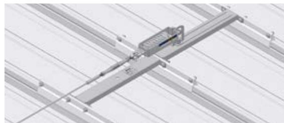
end bracket fall absorption with spring pre-tension (approx. 0.75 kN) and indicator fixation
