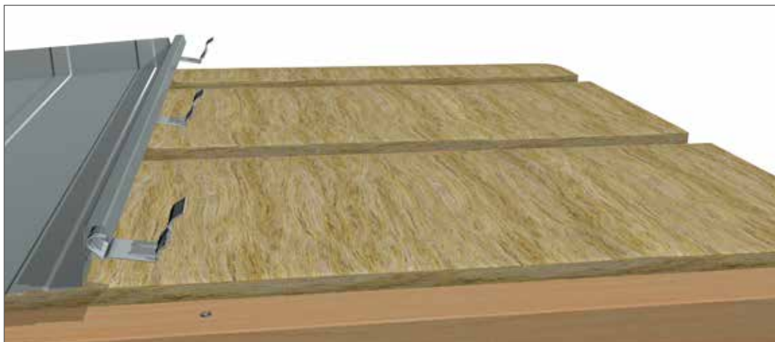
The position of the sliding clips (standard clips/directional clips) is determined by the profiled sheet width.
