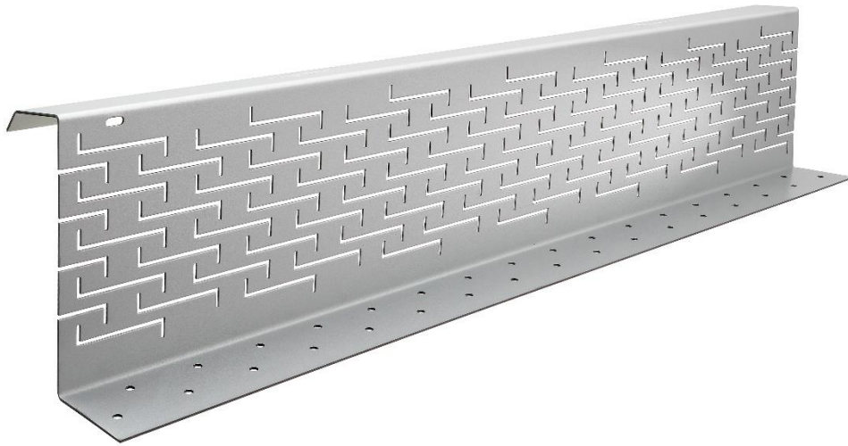
The new Thermo-Z spacer profile achieves optimal U-values. Multiple rows of staggered elongated holes redirect heat flow, effectively reducing thermal bridging. Photo: Zambelli Holding GmbH
